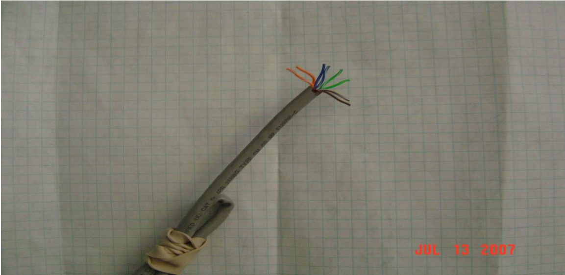
Figure-6: untwisting, straightening, and (somewhat) ordering the wires.
