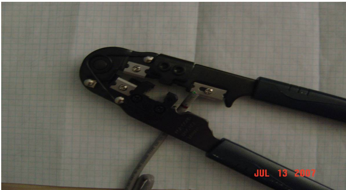
Figure-5: cutting the cable jacket. Rotate the wire not more than one time around.
