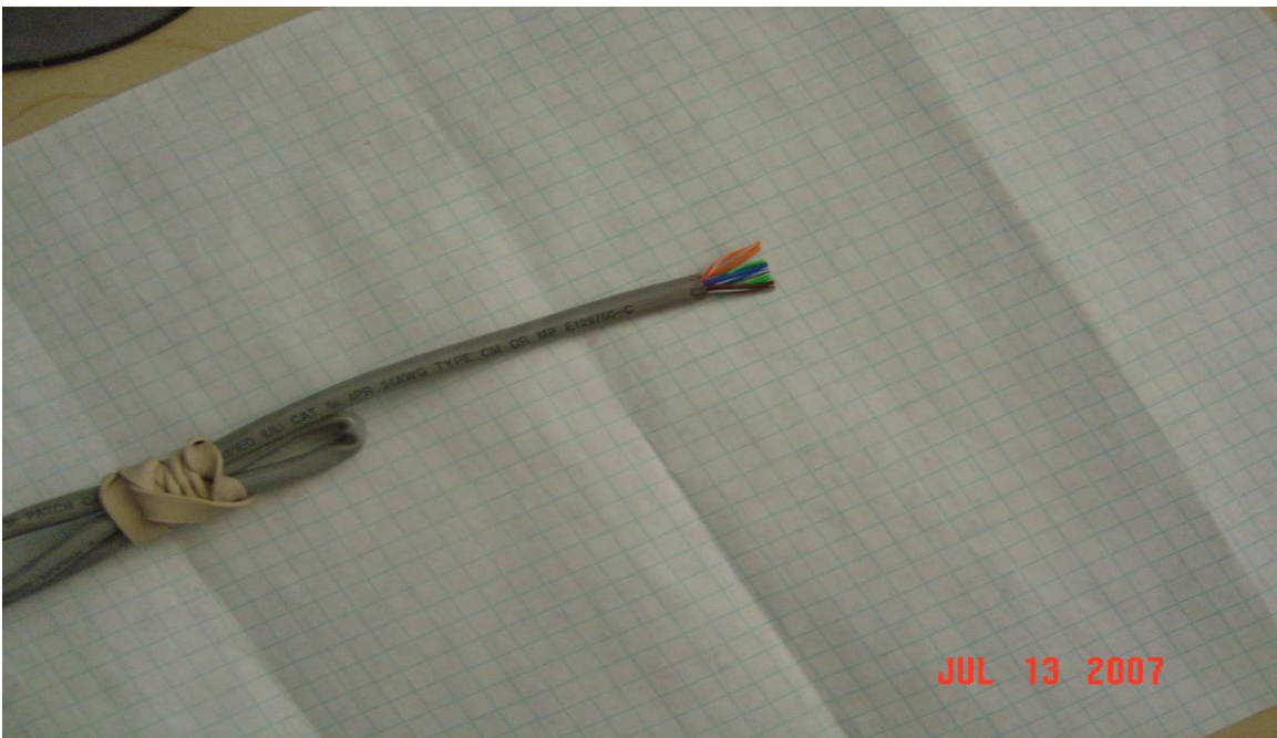
Figure 7: flatten and arrange the wires forward.
