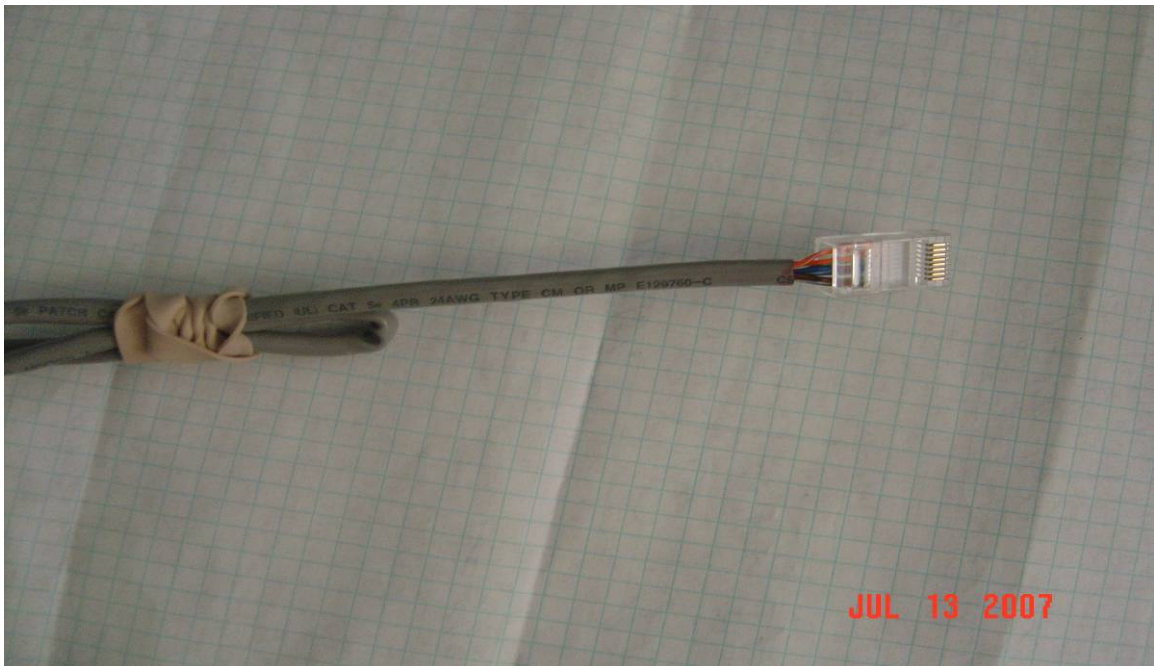
Figure-8: Working the wires into the RJ-45. Failure to position all wires correctly the first time is hardly a failure as insertion serves regardless to orient the wires to the RJ-45's wire guides. This photo shows initial insertion of the wires. Fully inserted the cable jacket will pass beneath the RJ-45's strain relief.
