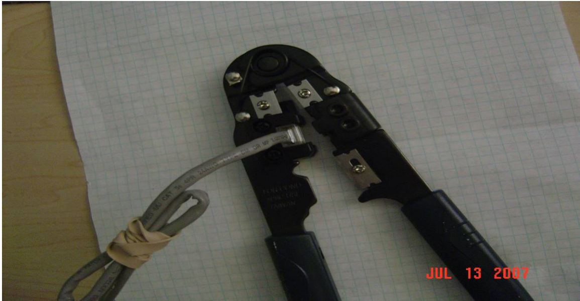
Figure-9: crimp city. The tool is designed to allow you to give it everything you got, so please do. The tool should (and must) completely close.
