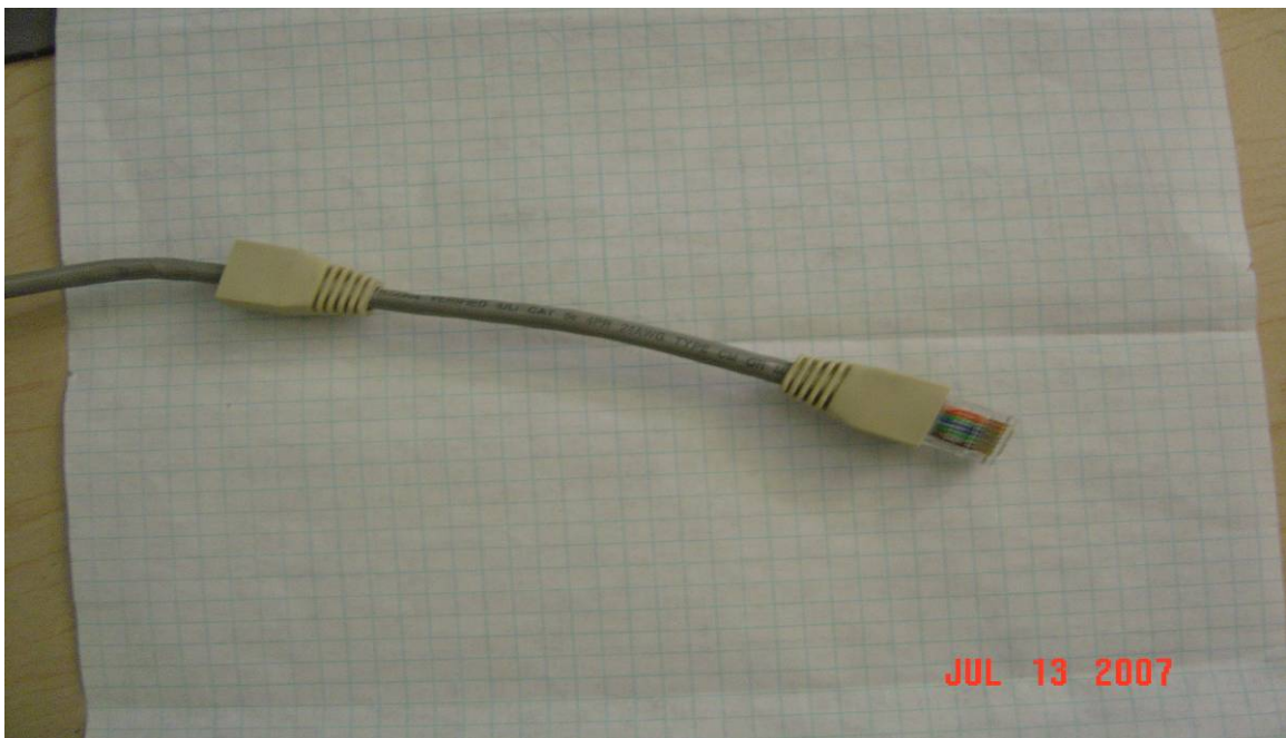
Figure-10: one side completed, and both anti-snag boots installed.
